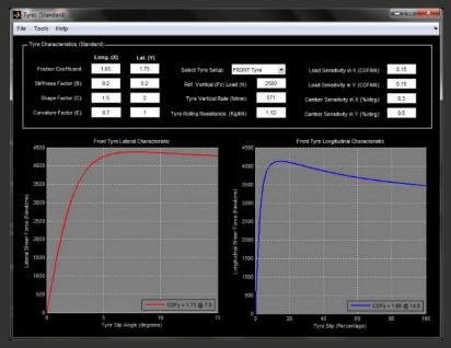
The vehicle definition is comprehensive for advanced users, for example it includes a non-linear tyre model which is based on Pacejkas 'Magic Formula' construction.
