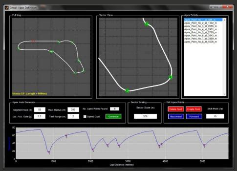
The Circuit Tool deconstructs the imported data and re-constructs a file which is suitable for use with the simulation algorithm. In doing so it breaks the path down into discrete sections over which the solution algorithm works.
