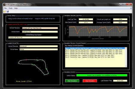
Running alongside the vehicle and/or circuit tools the vehicle or path parameters can be easily adjusted and the simulation rerun quickly without the need to generate and save completely new vehicle or path (circuit) files.
