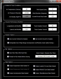
The 'Solver Options' and 'Solution Setup' menus allow the user to specify simulation parameters for convergence and resolution as well as ambient conditions, overall track grip levels, performance parameters (extent to which the peak tyre performance is utilised) etc. Here the user also has options on how the software saves data files for post processing and what data is to be output to those files.
