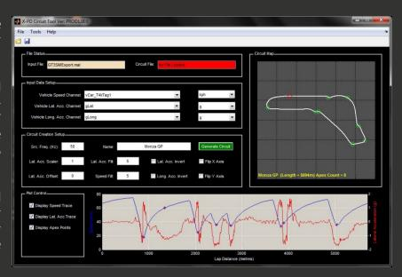
The resultant path (circuit) file, once complete, can be saved for direct use in the LapSIM solver and re-opened for editing if required.
