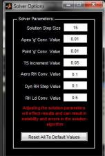
The solution algorithm itself is iterative around the lap over a user defined step size (increments of distance), allowing a choice between a high resolution and level of absolute accuracy (short steps) or a more efficient (and rapid) simulation speed (larger distance increments between calculations). The algorithm does also dynamically adjust resolution to capture high frequency events when they occur to achieve the best compromise.
